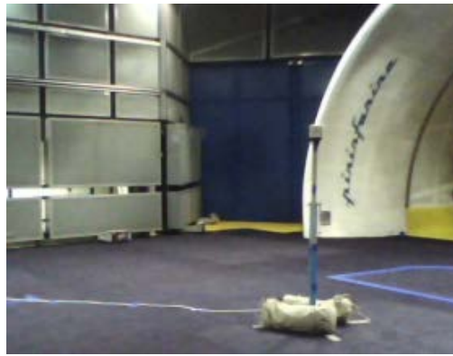
Figure 8. A speaker in the wind tunnel producing white noise sound.
