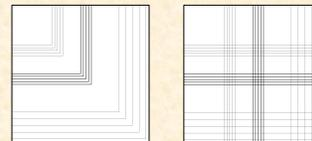
These patterns were irradiated at 10 different doses on 4 samples of each formulation. The scan resolution was 1024 pixels, the scan size was 1000  $\mu\text{m}$ , and therefore the developed line widths were thicker than the pixel size due to our beam spot size. The samples were exposed at doses from 100 to 640  $\text{nC}/\text{mm}^2$ . Top-down SEM images have been done from both resist formulations on all irradiations.
