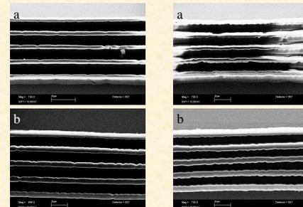
Representative results in case of PEB at 100°C for 8 min. The resist A (above) needs high dose (344  $\text{nC}/\text{mm}^2$ ) in order to resolve structures as small as 5  $\mu\text{m}$ . Moreover, this resist exhibits swelling and adhesion problems when it is developed for long times. Resist B (below) shows much better results at smaller exposure dose (238  $\text{nC}/\text{mm}^2$ ) without exhibiting adhesion problems.
