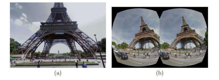
Figure 1.9: A simple VR experience that presents Google Street View images through a VR headset: (a) A familiar scene in Paris. (b) Left and right eye views are created inside the headset, while also taking into account the user's looking direction.
