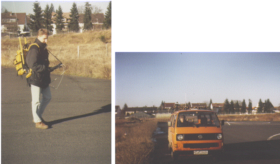
Figure 4 Roving Site Mounted on a Backpack and on a Van
